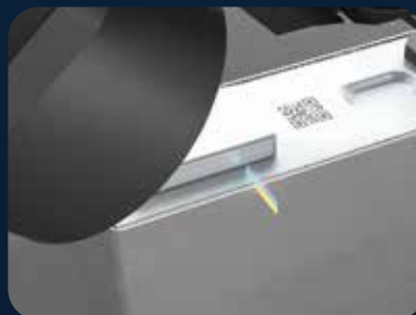
Weld seam inspection (tab, liquid injection port, etc.)
